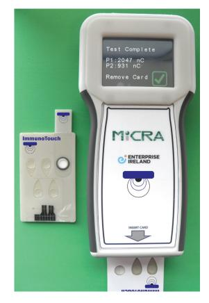
The testing kit enables rapid and quantitative measurement of anti-Fasciola (liver fluke) antibodies in milk and sera.
