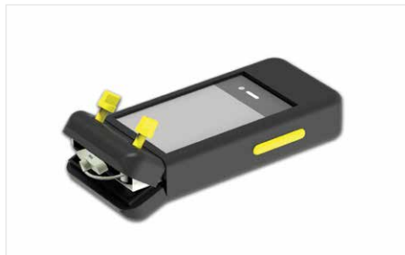
2. Connect the 30 pin connector, enabling the app to change the VHF channel and charge the phone.
